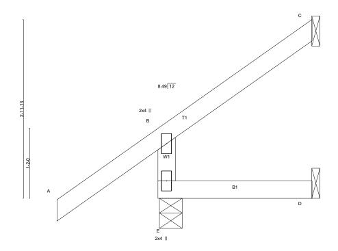
2-6-8 LOADING (psf) SPACING-CSI. DEFL. **PLATES GRIP** 2-0-0 in (loc) I/defl I/d 1.15 TC BC 244/190 Plate Grip DOL Vert(LL) -0.00 TCLL 20.0 0.24 D-E >999 240 MT20 **TCDL** 10.0 Lumber DOL 1.15 0.08 Vert(CT) -0.00 D-E >999 180 **BCLL** 0.0 Rep Stress Incr YES WB 0.00 Horz(CT) 0.01 С n/a n/a **BCDL** 10.0 Code IRC2015/TPI2014 Matrix-MR Weight: 13 lb FT = 20%
