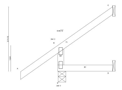
2-6-2 LOADING (psf) SPACING-CSI. DEFL. **PLATES GRIP** 2-0-0 in (loc) I/defl I/d 1.15 TC BC 244/190 Plate Grip DOL Vert(LL) -0.00 TCLL 20.0 0.25 D-E >999 240 MT20 **TCDL** 10.0 Lumber DOL 1.15 0.08 Vert(CT) -0.00 D-E >999 180 **BCLL** 0.0 Rep Stress Incr YES WB 0.00 Horz(CT) 0.01 С n/a n/a **BCDL** 10.0 Code IRC2015/TPI2014 Matrix-MR Weight: 13 lb FT = 20%
