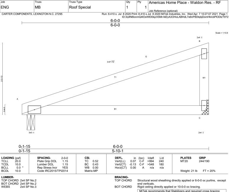
MiTek recommends that Stabilizers and required cross bracing be installed during truss erection, in accordance with Stabilizer Installation guide.
