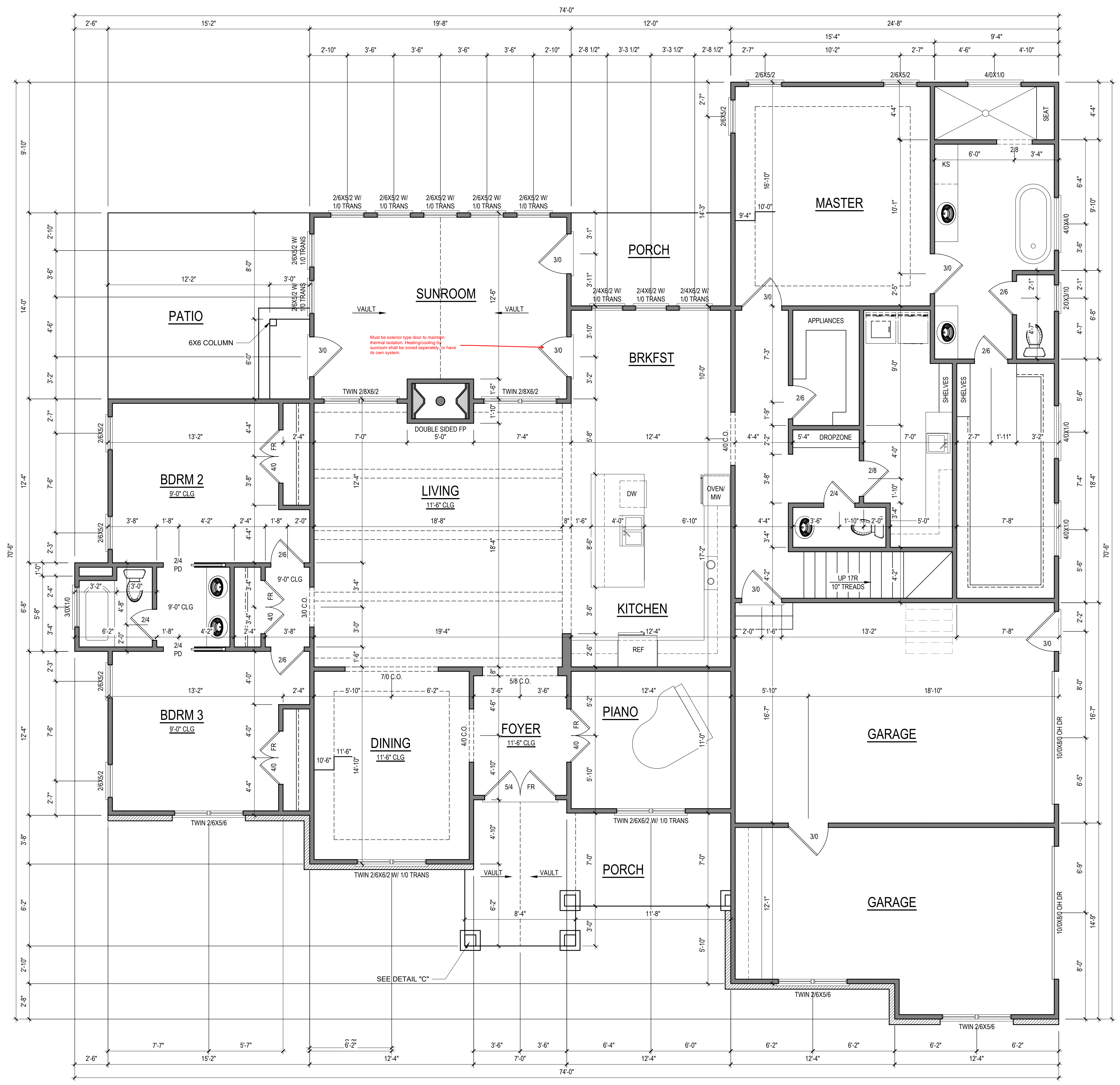
FIRST FLOOR PLAN 1/4" = 1'-0" CEILING HGT. = 10'-0"
