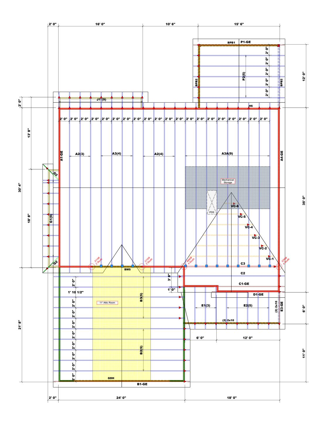
Truss Placement Plan SCALE: 3/16" = 1'-0"
