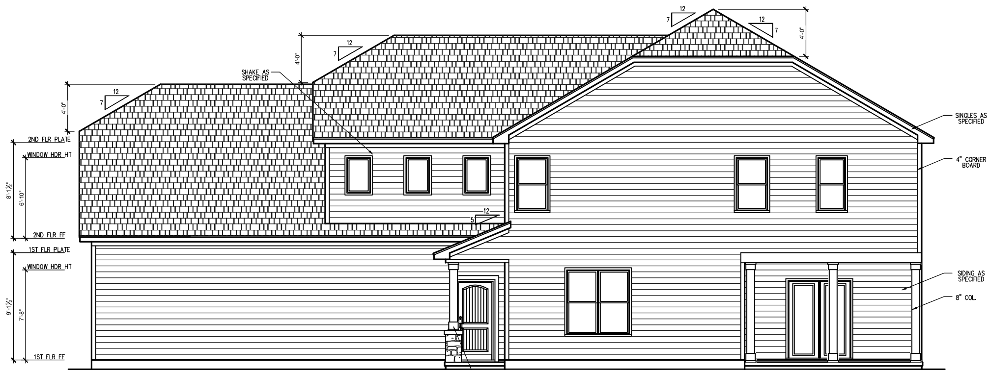
RIGHT SIDE ELEVATION - HERITAGE EUROPEAN SCALE: 1/4" = 1'-0" ON 22x34, 1/8" = 1'-0" ON 11x17 MONOLITHIC SLAB
