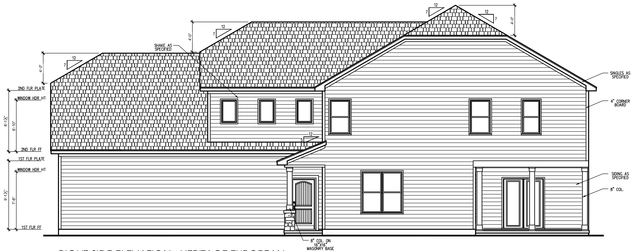
RIGHT SIDE ELEVATION - HERITAGE EUROPEAN SCALE: 1/4" = 1'-0" ON 22x34, 1/8" = 1'-0" ON 11x17 MONOLITHIC SLAB
