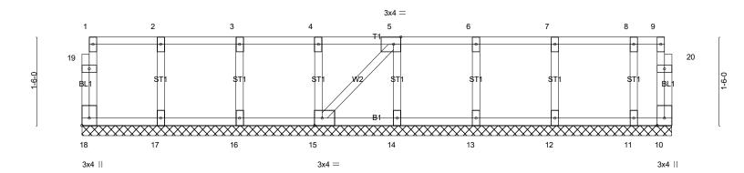
9-11-12 Plate Offsets (X,Y)-- [5:0-1-8,Edge], [15:0-1-8,Edge], [18:Edge,0-1-8] LOADING (psf) SPACING-CSI. DEFL PLATES **GRIP** 2-0-0 in (loc) I/defl I/d **TCLL** 40.0 Plate Grip DOL 1.00 TC 0.06 Vert(LL) n/a n/a 999 MT20 244/190 TCDL 10.0 Lumber DOL 1.00 вс 0.01 Vert(CT) n/a n/a 999 YES WB 0.03 0.00 **BCLL** 0.0 Rep Stress Incr Horz(CT) 10 n/a n/a BCDL Code IRC2018/TPI2014 Weight: 52 lb FT = 0%F, 0%E Matrix-SH
