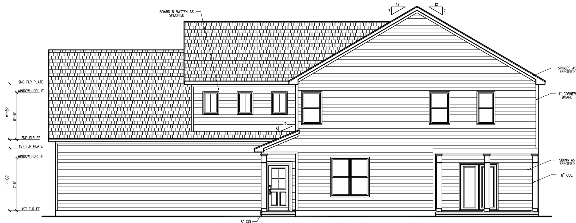
RIGHT SIDE ELEVATION - HERITAGE FARMHOUSE SCALE: 1/4" = 1'-0" ON 22x34, 1/8" = 1'-0" ON 11x17 MONOLITHIC SLAB
