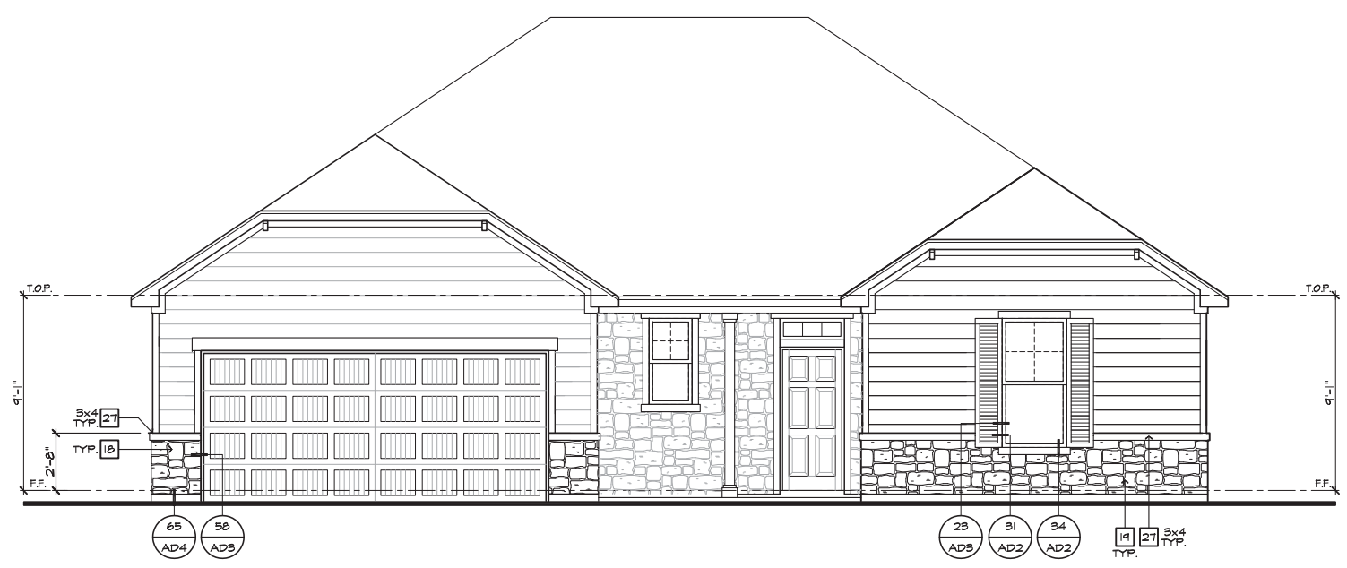
FRONT ELEVATION 'D' W/ STONE AT OPTIONAL 9'-1" PLT. HGT. SCALE 1/4"=1'-0" (22'x34') - 1/8"=1'-0" (11'x17')
