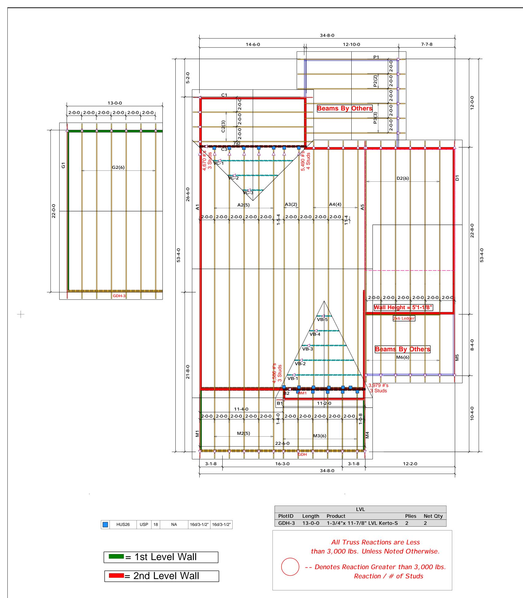
Truss Placement Plan SCALE: 1/4"=1' = Indicates Left End of Truss
