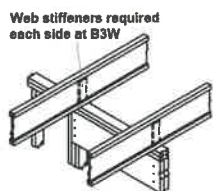
B3 B3W Blocking panels may be required with shear walls above or below (See detail B1).
