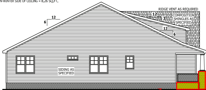
LEFT SIDE ELEVATION SCALE 1/8" = 1'-0"
