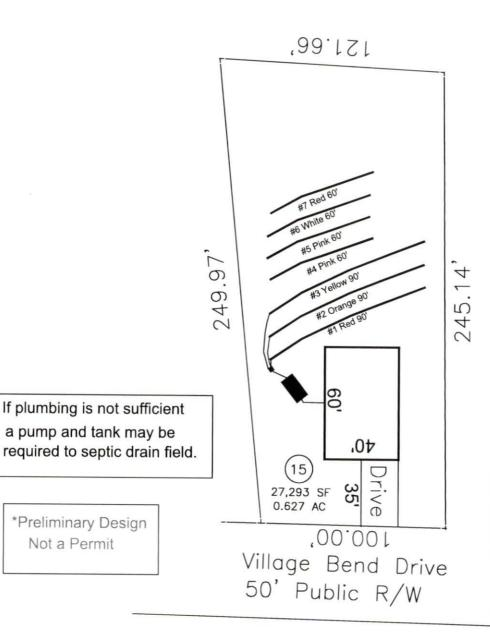
System: Gravity to D-Box Lines: 1-3 (270') 0.325 LTAR 24" Trench Bottom Accepted Status System Repair: Gravity to D-Box Lines: 4-7 (200') 0.325 LTAR 24 Trench Bottom T&J Panel - 50% Reduction System
