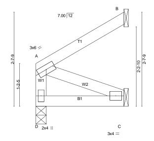
SPACING-LOADING (psf) GRIP CSI. DEFL. **PLATES** 2-0-0 (loc) I/defl L/d Plate Grip DOL TCLL 20.0 1.15 TC 0.09 Vert(LL) -0.00 C-D >999 360 MT20 244/190 вС **TCDL** 10.0 Lumber DOL 1.15 0.06 Vert(CT) -0.00 C-D >999 240 **BCLL** 0.0 \* Rep Stress Incr YES WB 0.03 Horz(CT) -0.00 n/a \*\*\*\* n/a Code IRC2015/TPI2014 Matrix-MP Wind(LL) 0.00 D 240 Weight: 13 lb FT = 20% **BCDL** 10.0
