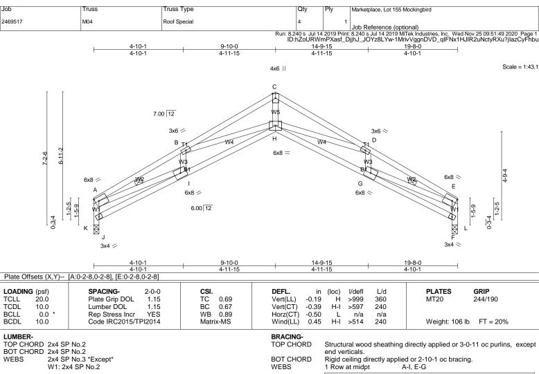
MiTek recommends that Stabilizers and required cross bracing be installed during truss erection, in accordance with Stabilizer Installation guide.
