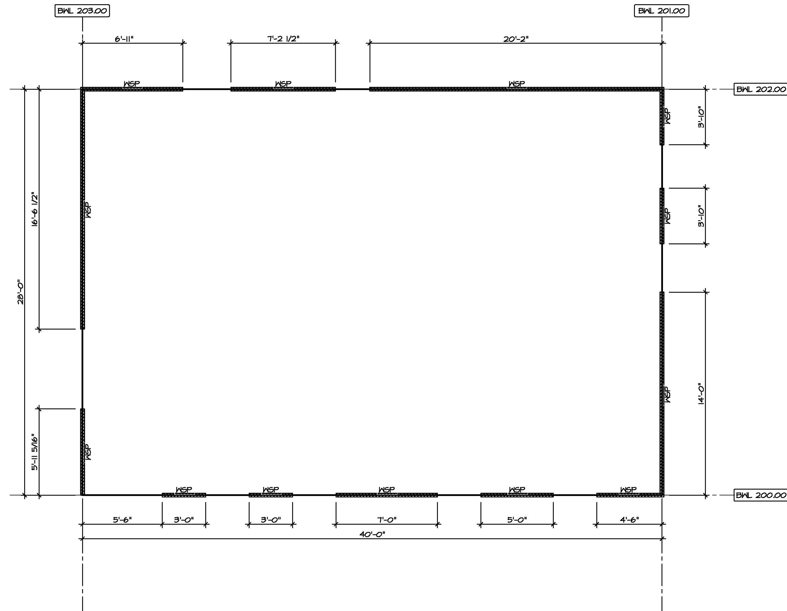
2 SECOND FLOOR BRACED WALL DETAIL SCALE: 1/4" = 1'-0"
