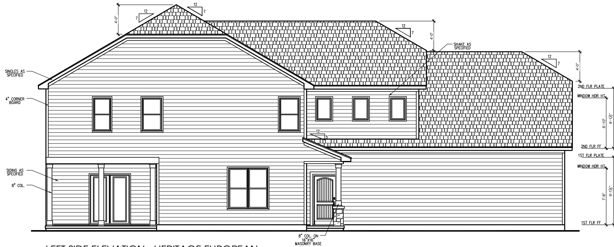
LEFT SIDE ELEVATION - HERITAGE EUROPEAN SCALE: 1/4" = 1'-0" ON 22x34, 1/8" = 1'-0" ON 11x17 MONOLITHIC SLAB
