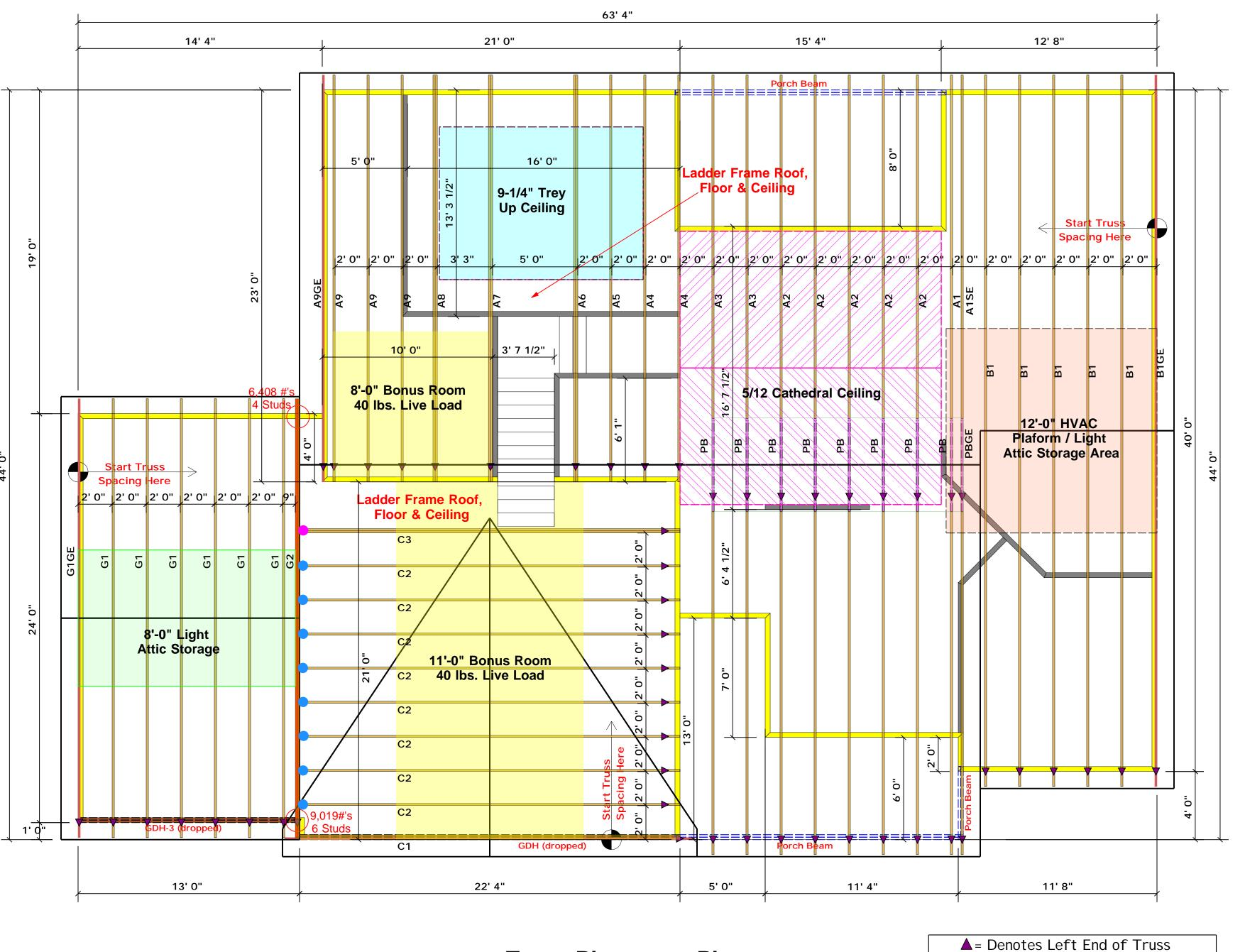
Truss Placement Plan SCALE: 1/4" = 1'0"
