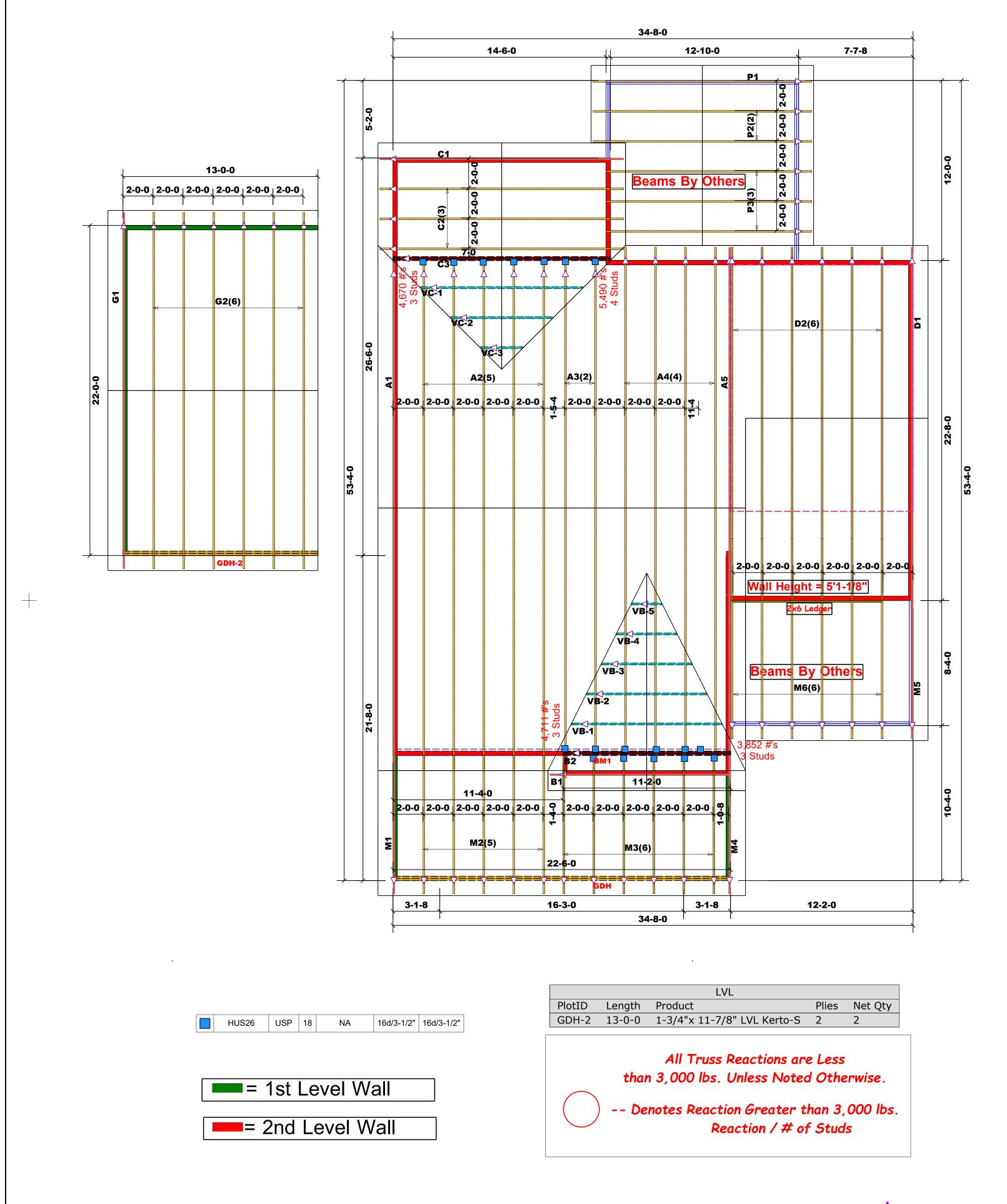
Truss Placement Plan SCALE: 1/4"=1' = Indicates Left End of Truss
