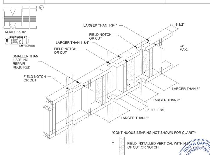
FLOOR GABLES(S) (LADDER TRUSSES) ARE CONVENTIONAL WALLS WITH CONNECTOR PLATES PER ANSI/TPE SECTION 6.6 AND USED IN CONVENTIONAL WALL FRAMING MEETING IRC SECTION R602. REFER TO MITEK/TRENCO DESIGN DRAWING FOR MATERIAL SPECIFICATIONS.
