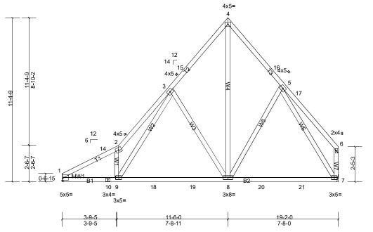
Loading (psf) **Spacing** 2-0-0 CSI **DEFL** (loc) I/defl L/d **PLATES GRIP** TCLL (roof) 20.0 Plate Grip DOL 1.15 TC 0.30 Vert(LL) -0.10 8-9 >999 240 MT20 244/190 1.15 -0.20 **TCDL** 10.0 Lumber DOL BC 0.45 Vert(CT) >999 180 8-9 **BCLL** 0.0 Rep Stress Incr YES WB 0.73 Horz(CT) 0.02 7 n/a n/a **BCDL** IBC2015/TPI2014 Weight: 136 lb FT = 20% 10.0 Code Matrix-MS
