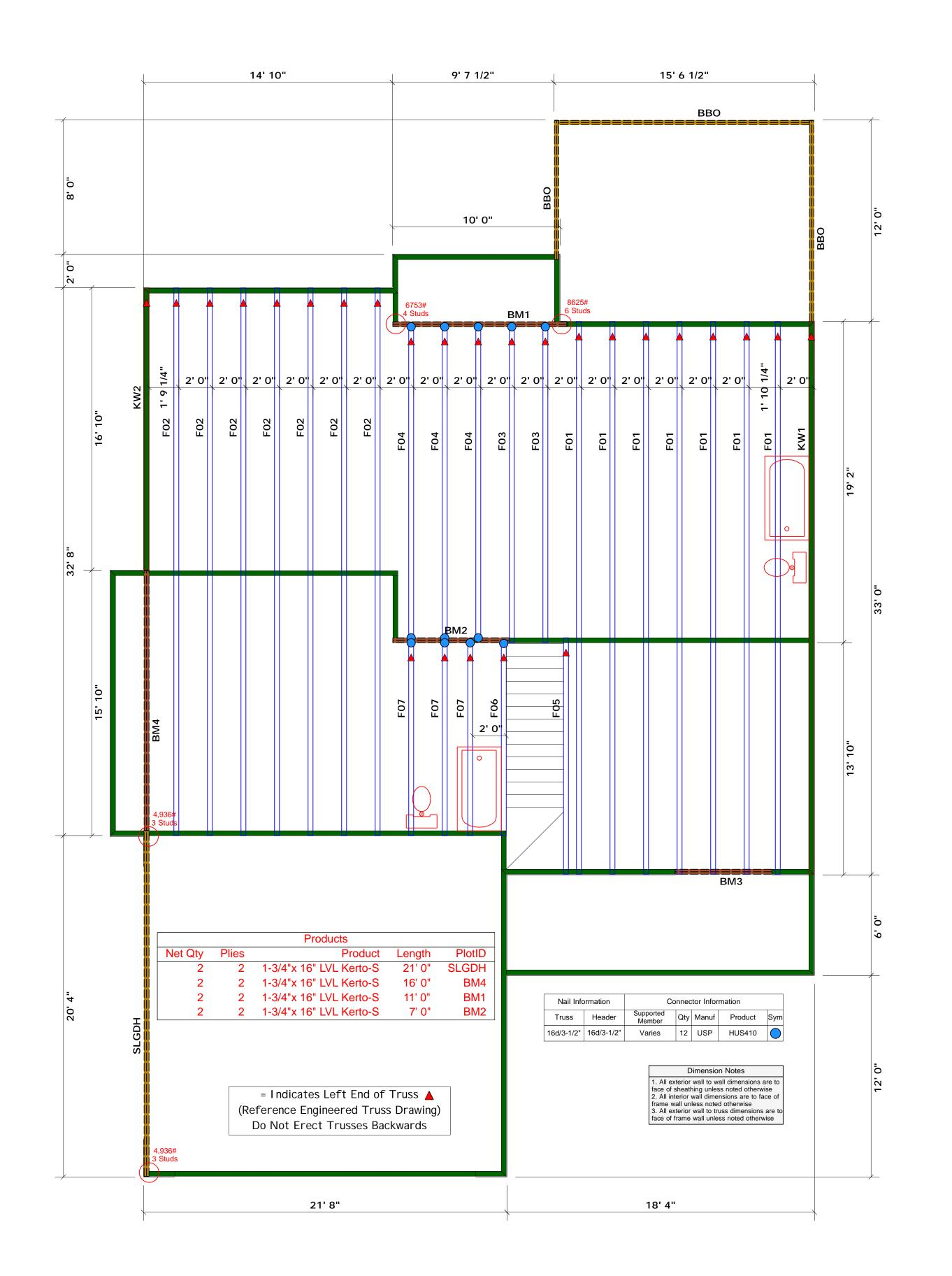
Truss Placement Plan SCALE: 1/4" = 1'
