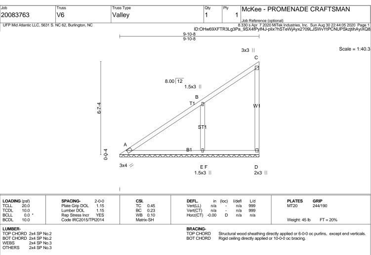
**REACTIONS.** (lb/size) A=175/9-10-8 (min. 0-1-8), D=96/9-10-8 (min. 0-1-8), E=471/9-10-8 (min. 0-1-8)
