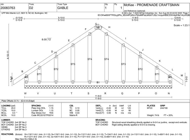
Max UpiritW=-67(LC 6), N=-48(LC 7), T=-59(LC 10), U=-33(LC 10), V=-87(LC 10), Q=-60(LC 11), P=-34(LC 11), O=-82(LC 11)
