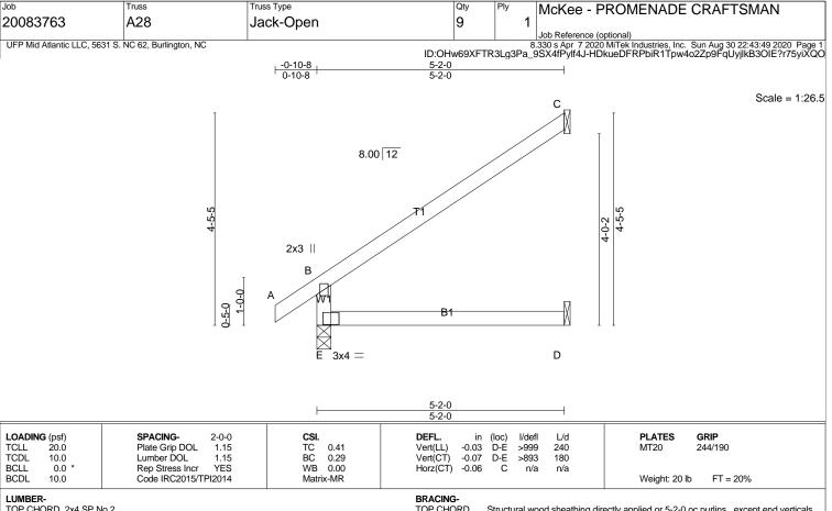
TOP CHORD 2x4 SP No.2 BOT CHORD 2x4 SP No.2 2x4 SP No.3 TOP CHORD BOT CHORD Structural wood sheathing directly applied or 5-2-0 oc purlins, except end verticals. Rigid ceiling directly applied or 10-0-0 oc bracing.
