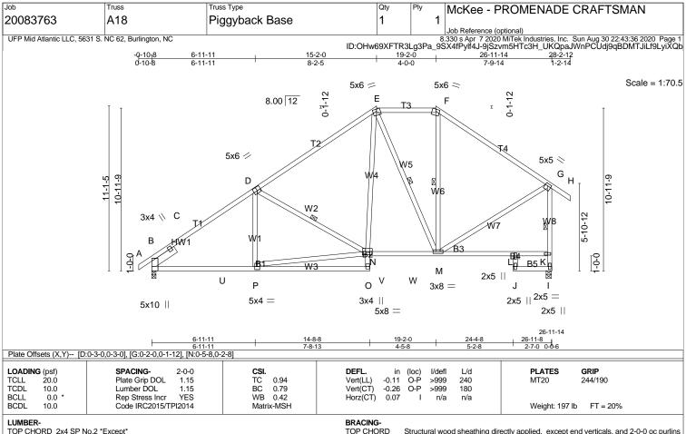
Structural wood sheathing directly applied, except end verticals, and 2-0-0 oc purlins
