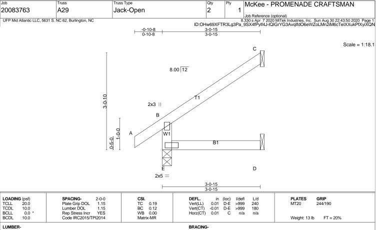
TOP CHORD 2x4 SP No.2 BOT CHORD 2x4 SP No.2 2x4 SP No.3 TOP CHORD BOT CHORD Structural wood sheathing directly applied or 3-0-15 oc purlins, except end verticals. Rigid ceiling directly applied or 10-0-0 oc bracing.
