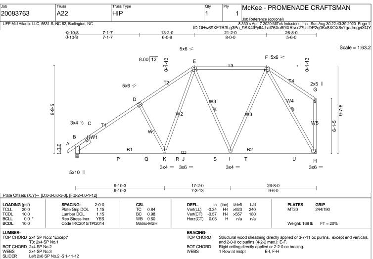
**REACTIONS.** (lb/size) B=1114/0-3-8 (min. 0-1-8), H=1060/Mechanical Max Horz B=311(LC 9)
