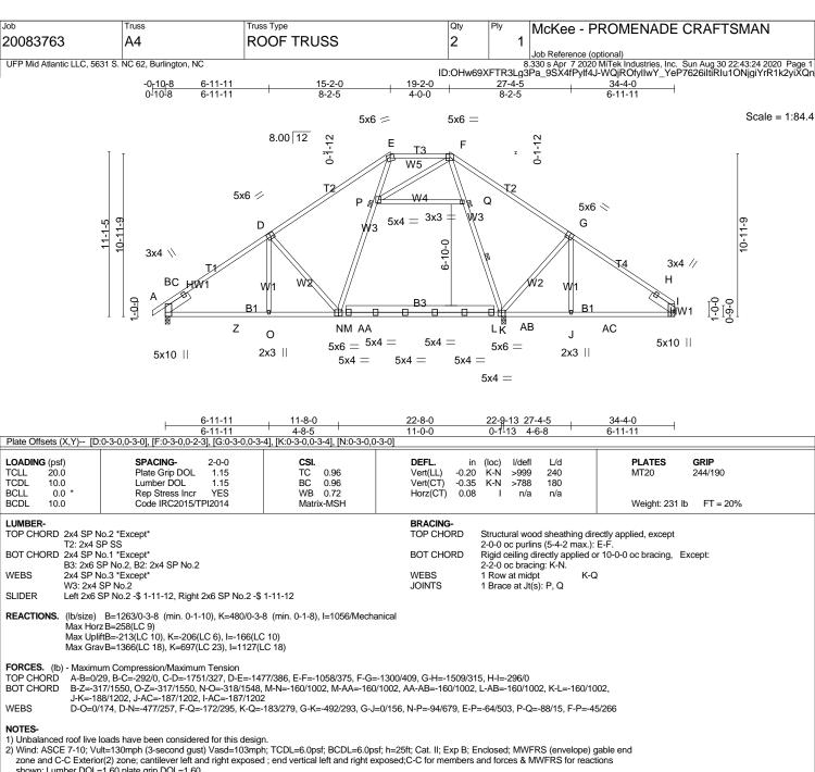
zone and C-C Exterior(2) zone; cantilever left and right exposed; end vertical left and right exposed; C-C for members and forces & MWFRS for reactions shown; Lumber DOL=1.60 plate grip DOL=1.60
