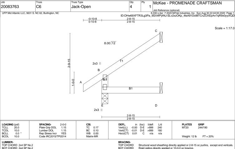
Structural wood sheathing directly applied or 2-8-15 oc purlins, except end verticals. Rigid ceiling directly applied or 10-0-0 oc bracing.
