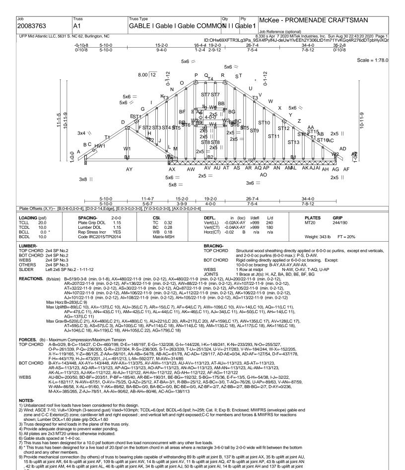
10) This truss is designed in accordance with the 2015 International Residential Code sections R502.11.1 and R802.10.2 and referenced standard ANSI/TPI.1.
