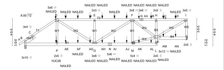
5-2-0 Plate Offsets (X,Y)-- [B:Edge,0-0-0], [D:0-4-12,Edge], [I:0-2-4,0-1-8] CSI. TC BC LOADING (psf) SPACING-2-0-0 DFFL. I/defl L/d **PLATES** GRIP (loc) Plate Grip DOL 0.54 244/190 TCLL 20.0 1.15 Vert(LL) 0.08 0 >999 240 MT20 TCDL 10.0 Lumber DOL 1.15 0.59 Vert(CT) -0.14 O-P >999 180 **BCLL** 0.0 Rep Stress Incr WB 0.58 NO Horz(CT) 0.02
