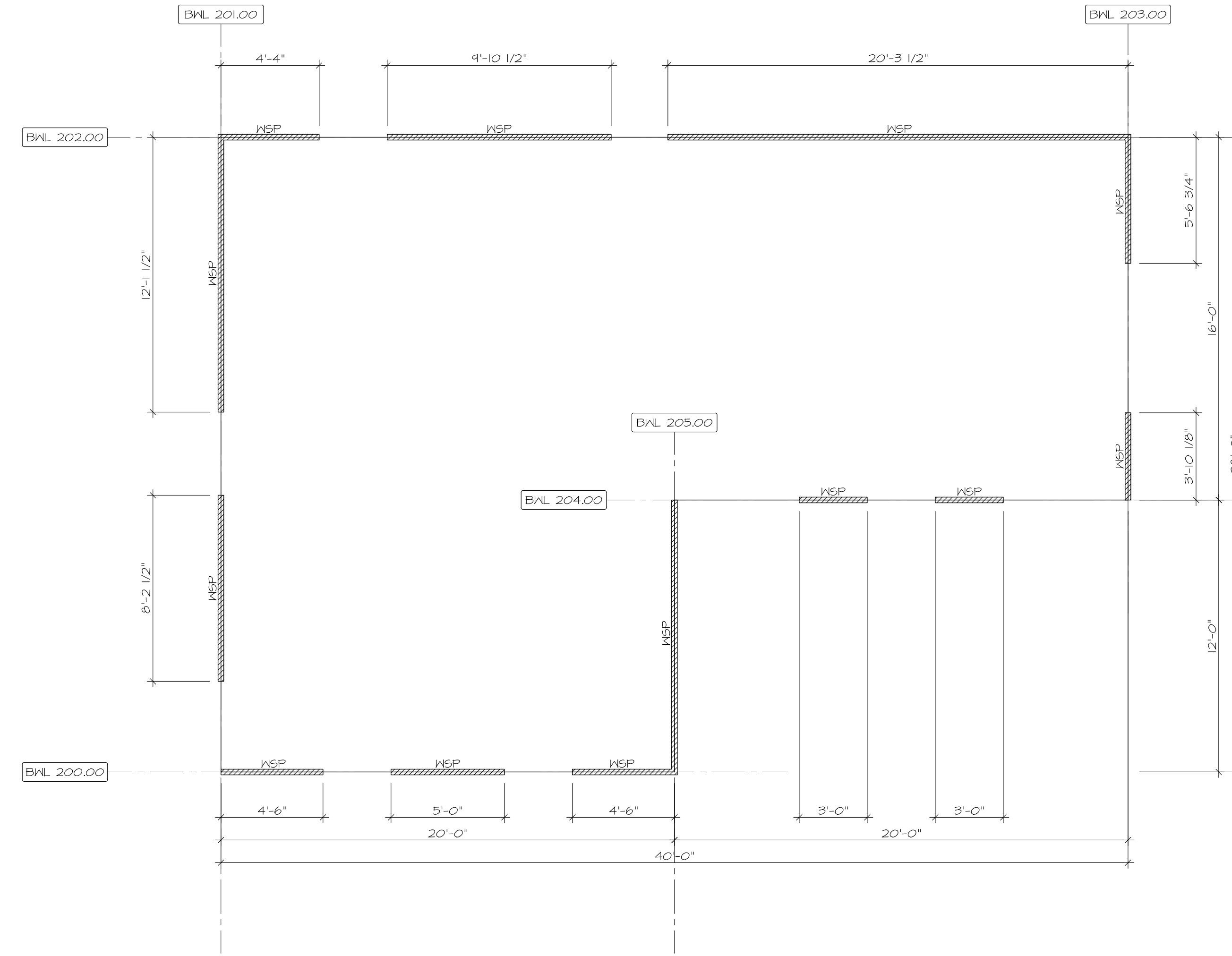
SECOND FLOOR BRACED WALL DETAIL SCALE: 1/4" = 1'-0"
