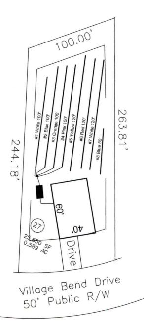
If plumbing is not sufficient a pump and tank may be required to septic drain field.
