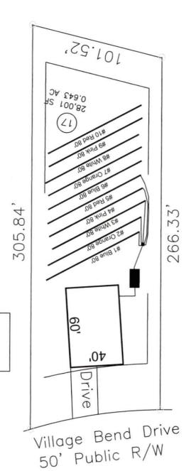
If plumbing is not sufficient a pump and tank may be required to septic drain field.
