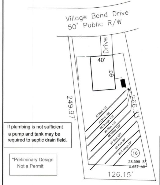
System: Gravity to D-Box Lines: 1-4 (400') 0.3 LTAR 24" Trench Bottom Accepted Status System Repair: Pressure Manifold Lines: 5-9 (400') 0.3 LTAR 24 Trench Bottom
