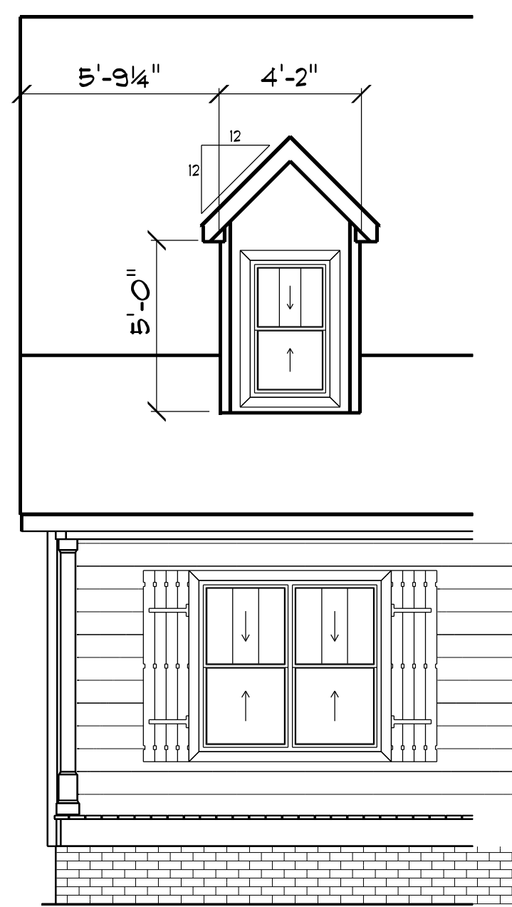
DORMER DETAIL PLAN SCALE: 1" = 1/4"
