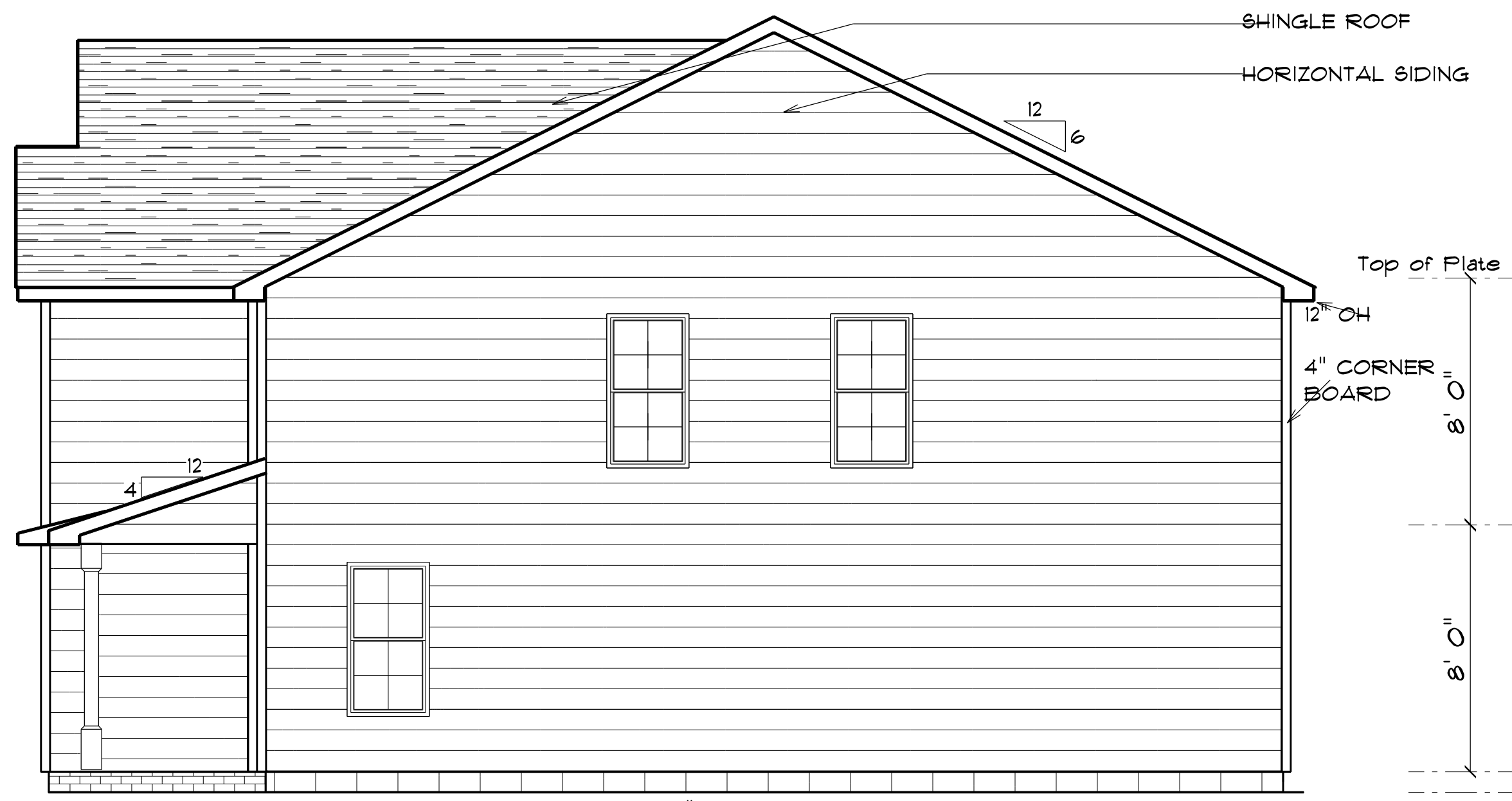
RIGHT ELEVATION SCALE: 1" = 1/4"
