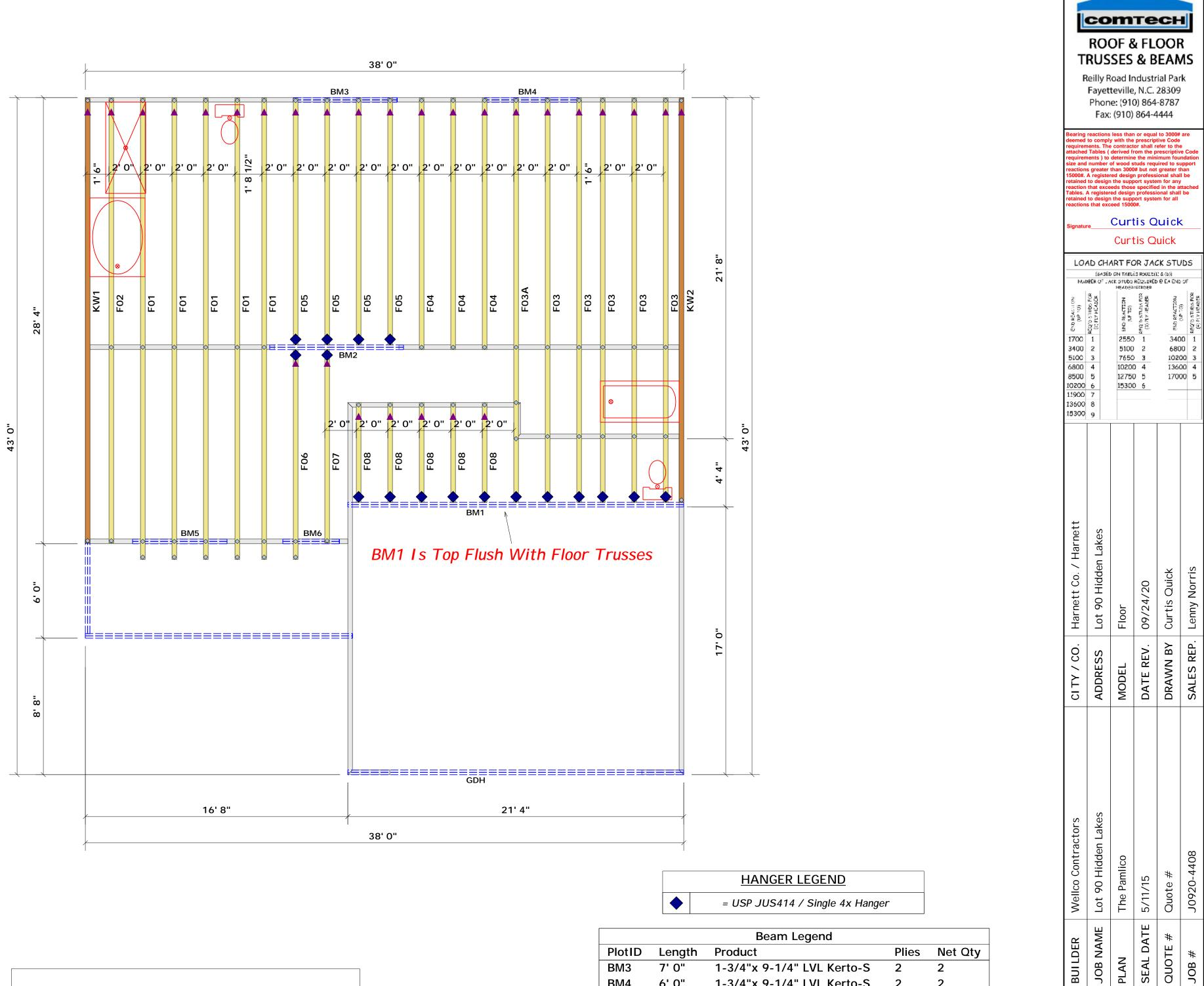
▲ = Denotes Left End of Truss (Reference Engineered Truss Drawing) Do Not Erect Trusses Backwards
