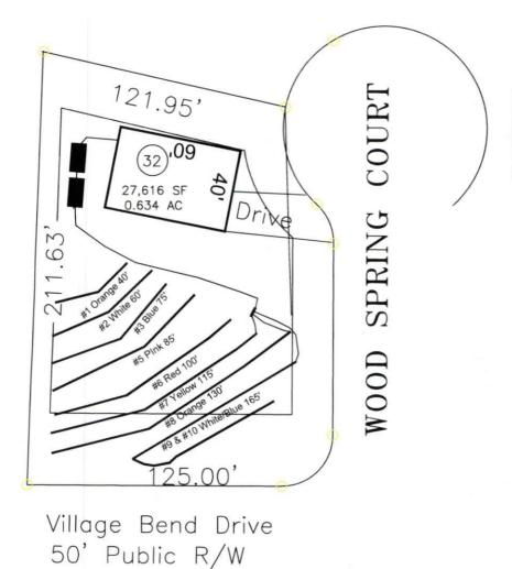
If plumbing is not sufficient a pump and tank may be required to septic drain field.
