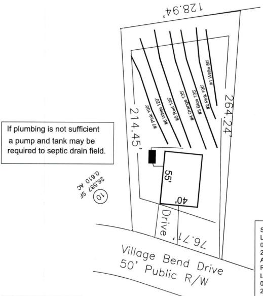
System: Gravity to D-Box Lines: 3-5 (405')
