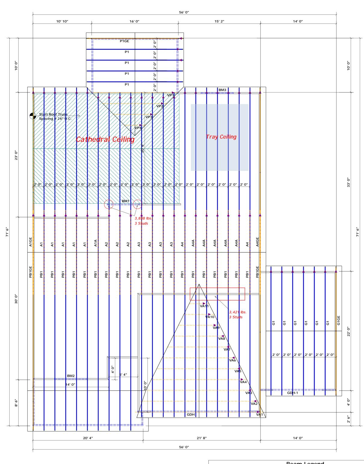
= Denotes Left End of Truss(Reference Engineered Truss Drawing)Do Not Erect Trusses Backwards
