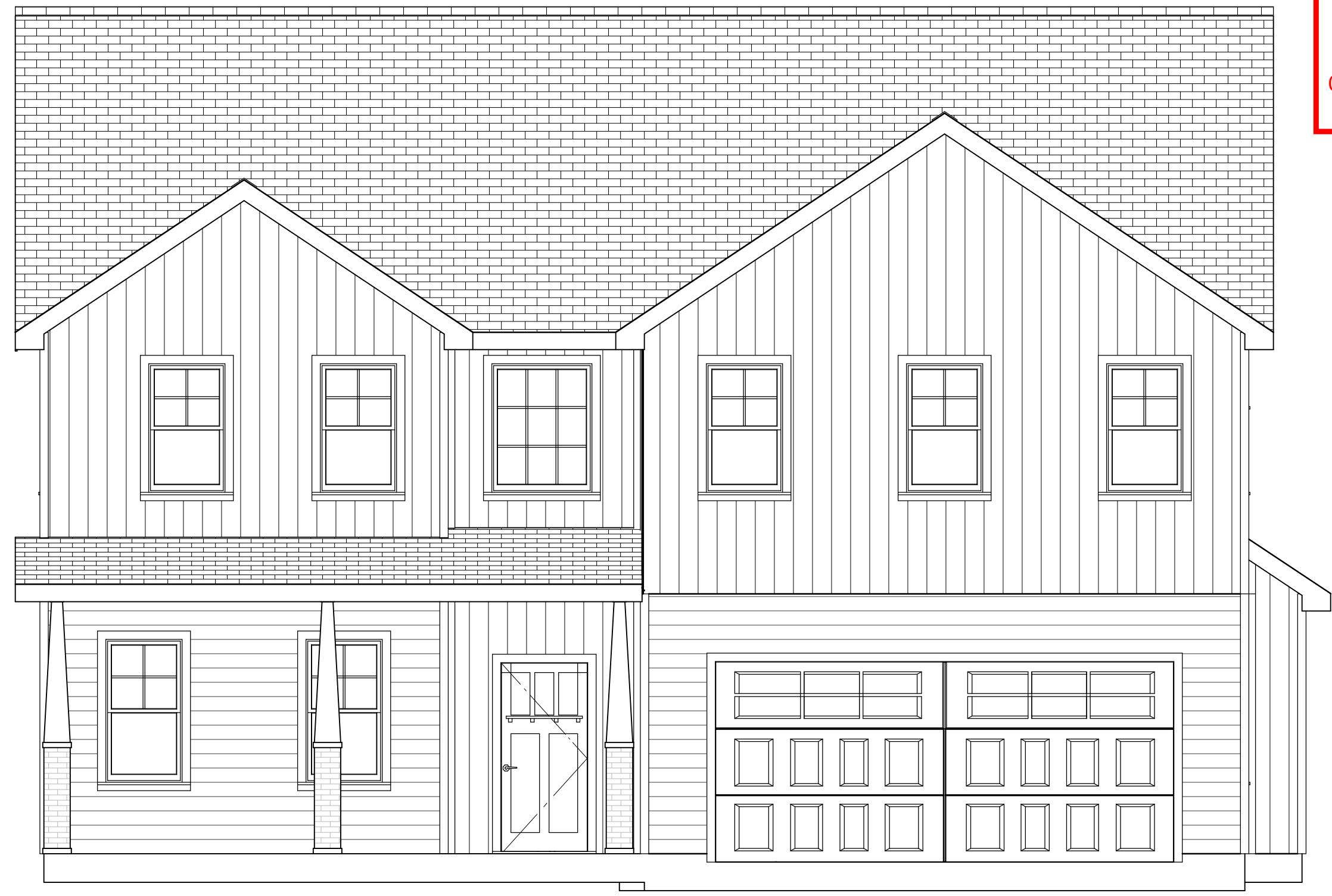
9'0" CEILING HEIGHT FIRST FLOOR (HEADER HEIGHT 7'6") 8'0" CEILING HEIGHT SECOND FLOOR (HEADER HEIGHT 7') FRONT ELEVATION Scale: 1/4" = 1'0" FRAME WINDOWS TO HEADER HEIGHT
