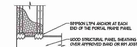
OVER RAISED WOOD FLOOR - FRAMING ANCHOR OPTION * APPLICABLE w/ GREATER THAN 12" KNEE WALL HEIGHTS IN ORAIL SPACE AND ABOVE FRAMED BASEMENT WALLS *
