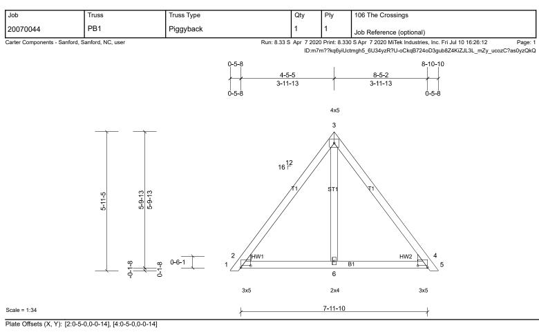
Loading (psf) Spacing 2-0-0 CSI DEFL l/defl L/d PLATES GRIP in (loc) TCLL (roof) 20.0 Plate Grip DOL 1.15 TC 0.31 Vert(LL) n/a n/a 999 MT20 244/190 Snow (Pf/Pg) 13.9/20.0 Lumber DOL 1.15 BC 0.32 Vert(CT) n/a 999 n/a TCDL 10.0 Rep Stress Incr YES WB 0.07 Horz(CT) 0.00 2 n/a n/a IRC2015/TPI2014 BCLL Matrix-MP 0.0 Code BCDL 10.0 Weight: 42 lb FT = 20%
