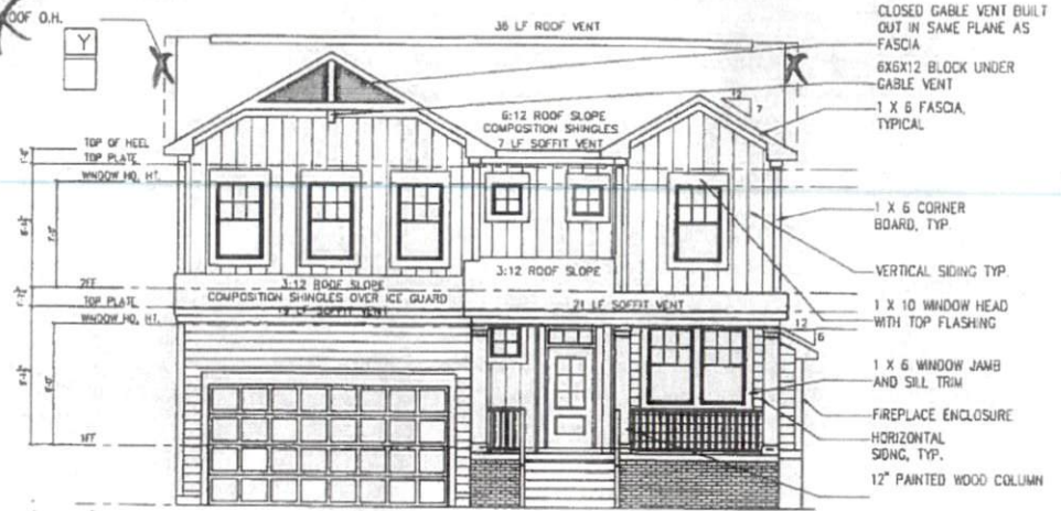
FRONT ELEVATION 'B' SCALE: 1/4"=1'-0" ON 22x34 AND 1/8"=1'-0" ON 11x17
