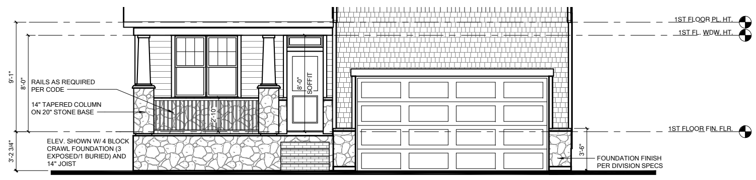
FRONT ELEVATION 'CRAFTSMAN' W/ CRAWL SPACE 3 1/4" = 1'-0" AT 22"X34" LAYOUT 1/8" = 1'-0" AT 11" X 17" LAYOUT
