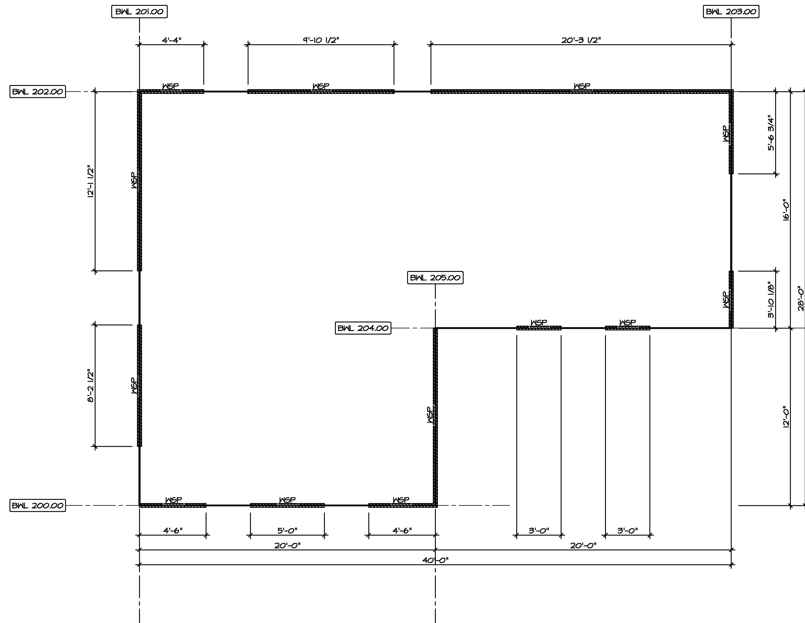
SECOND FLOOR BRACED WALL DETAIL 2 5-5 SCALE: 1/4" = 1'-0"
