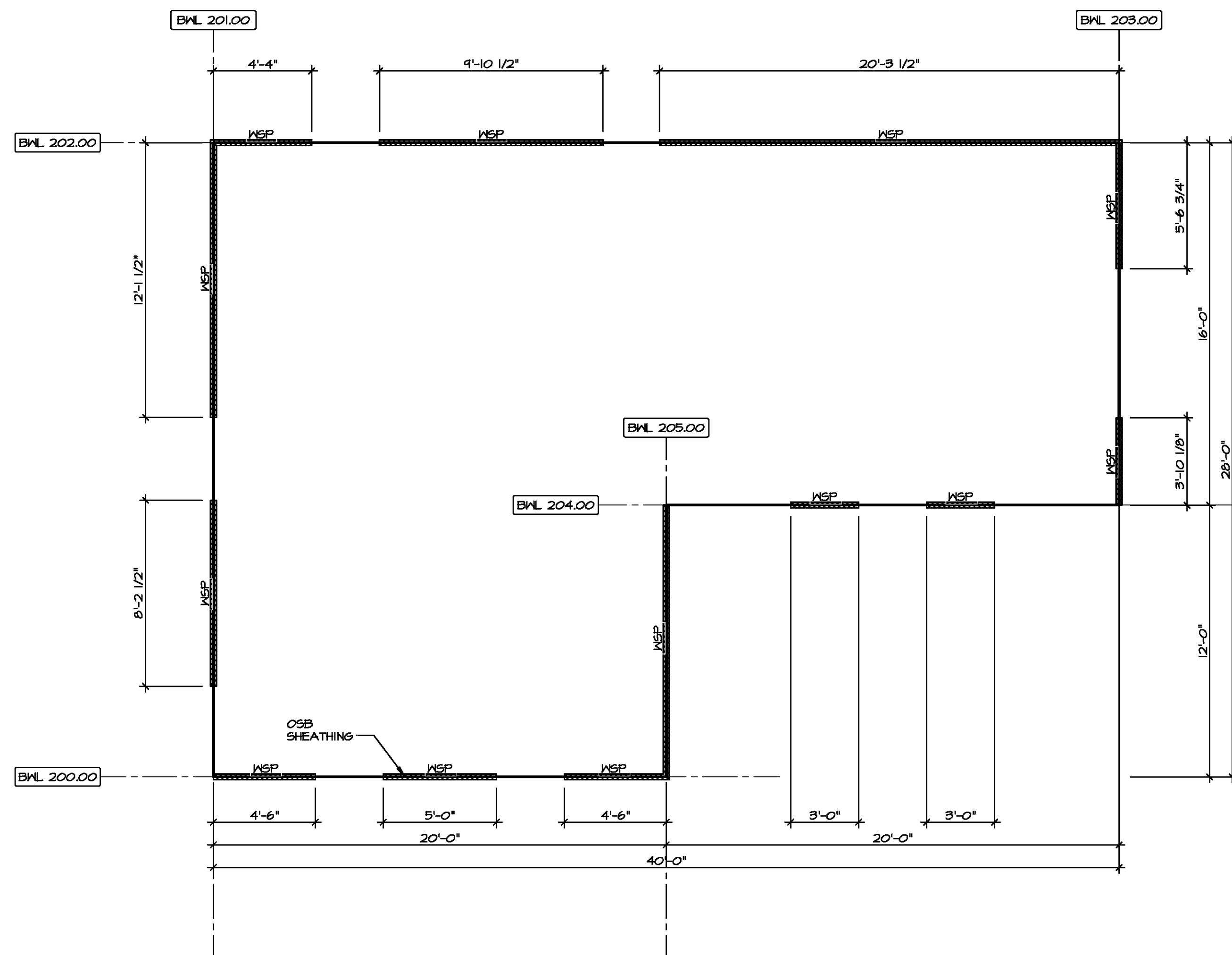
SECOND FLOOR BRACED WALL DETAIL SCALE: 1/4" = 1'-0"
