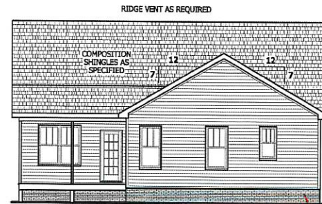
REAR ELEVATION SCALE 1/8" = 1'-0"
