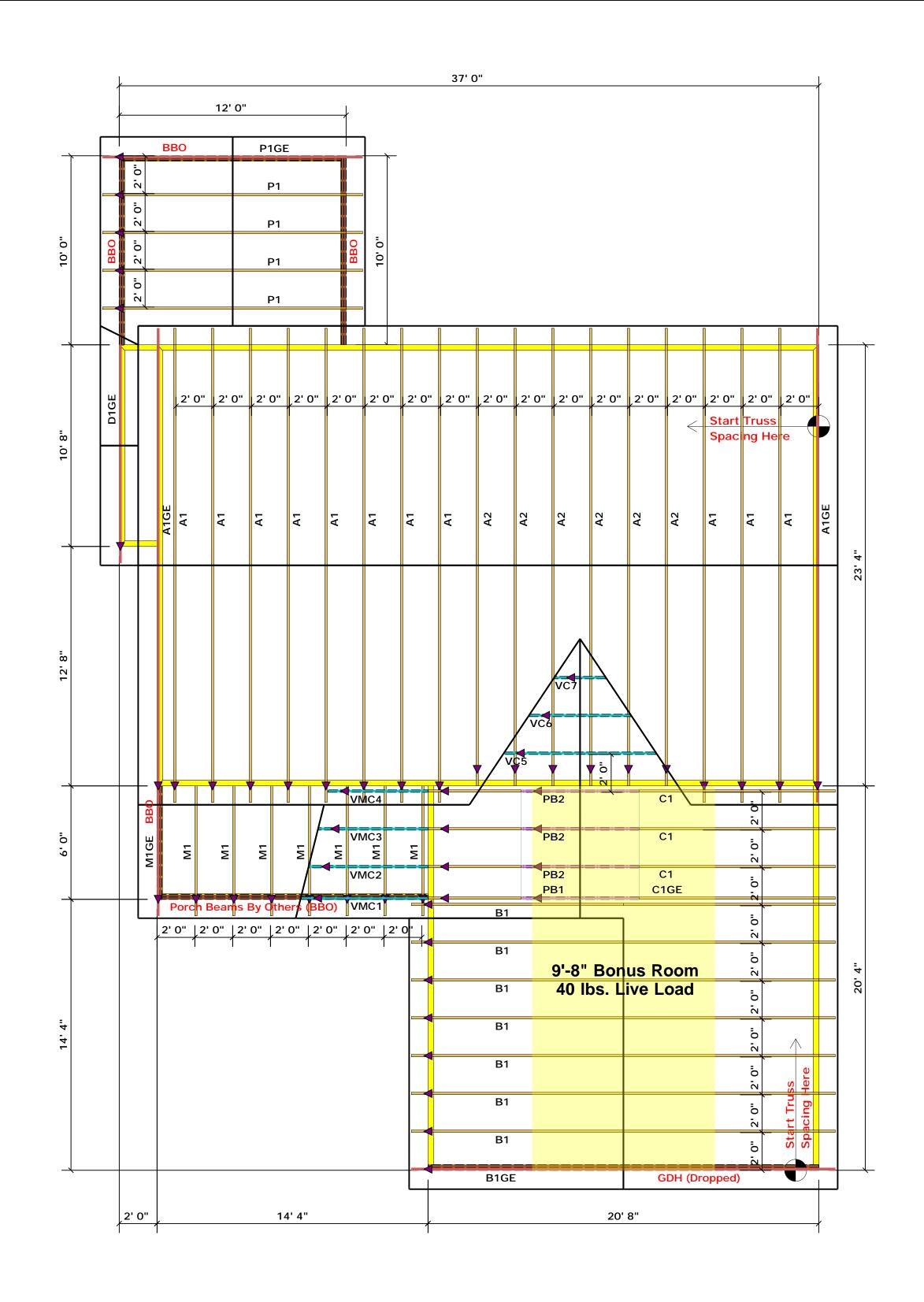
▲= Denotes Left End of Truss (Reference Engineered Truss Drawing)
