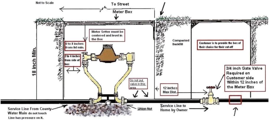
Cut-off valve requirement as specified in "AN ORDINANCE REGULATING THE USE OF WATER AND SEWER FACILITIES OPERATED BY THE COUNTY OF HARNETT, SECTION 32" AUTHORIZED BY THE HARNETT COUNTY BOARD OF COMMISSISSIONER, SEPTEMBER 6TH 1994
