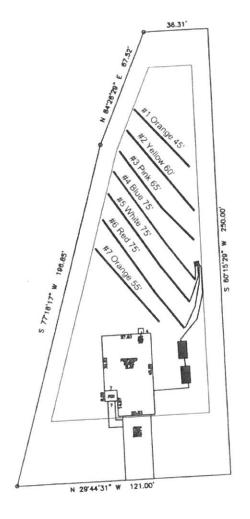
System: Pump to D-Box Lines: 4-6 (225') 0.4 LTAR 18-24" Trench Bottom Accepted Status System Repair: Pump to serial dist. Lines: 1-3, 7 (225')
