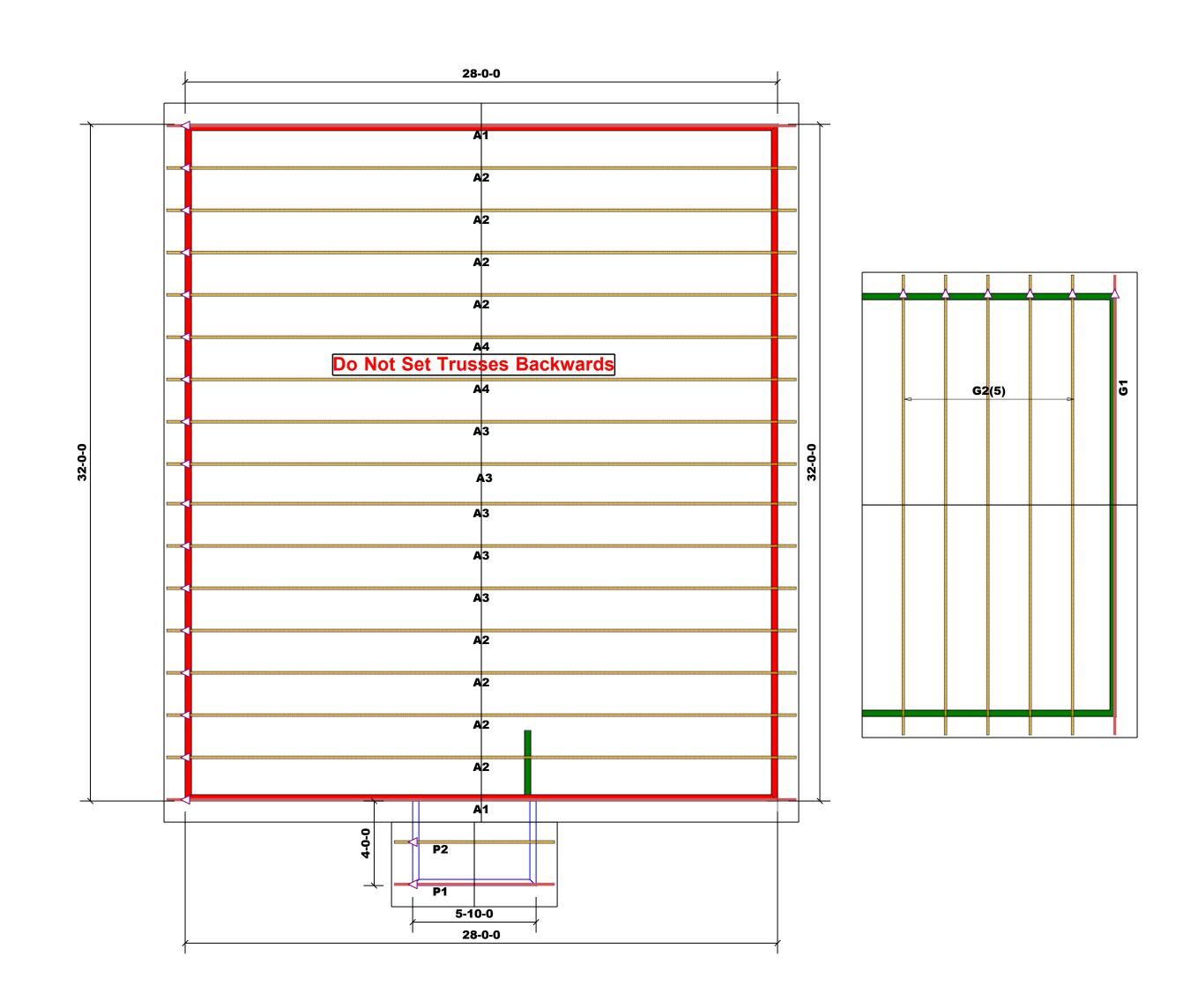
Truss Placement Plan SCALE: NTS
