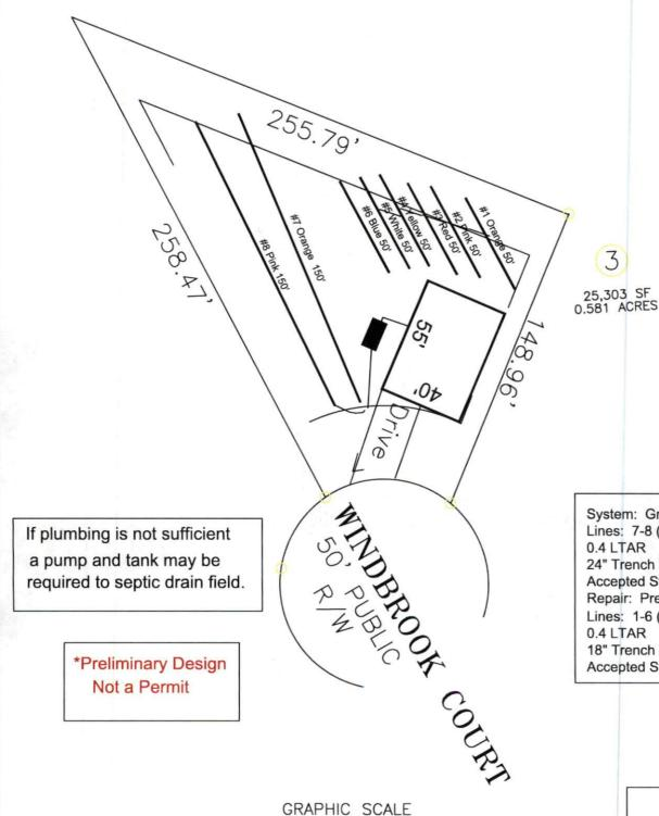
System: Gravity to D-Box Lines: 7-8 (300') 0.4 LTAR 24" Trench Bottom Accepted Status System Repair: Pressure Manifold Lines: 1-6 (300') 0.4 LTAR
