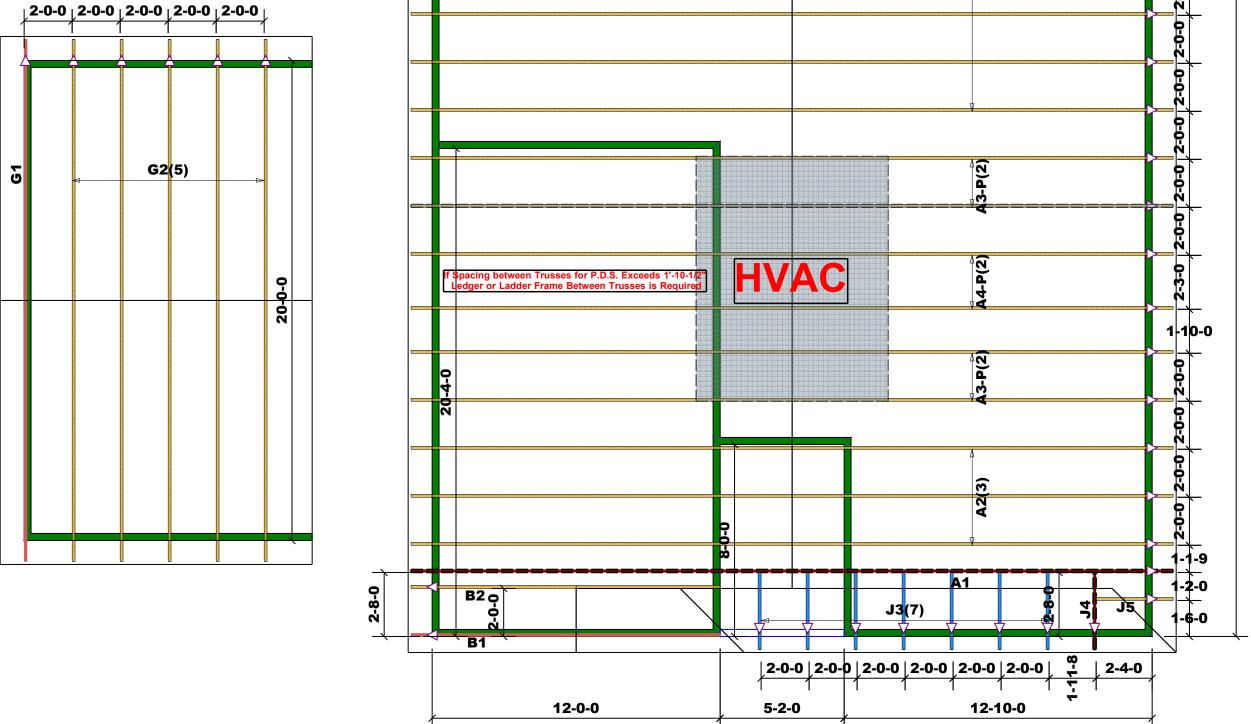
Truss Placement Plan SCALE: 1/4"=1'
