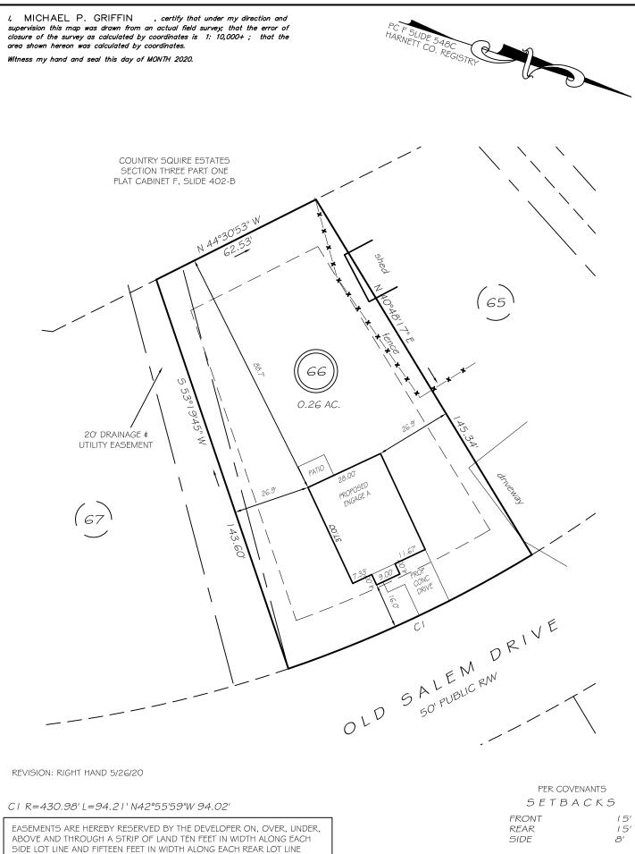
SIDE LOT LINE AND FIFTEEN FEET IN WIDTH ALONG EACH REAR LOT LINE AND FRONT LOT LINE FOR DRAINAGE, WATER AND SEWAGE INSTALLATION AND MAINTENANCE AND FOR OTHER UTILITY PURPOSES
