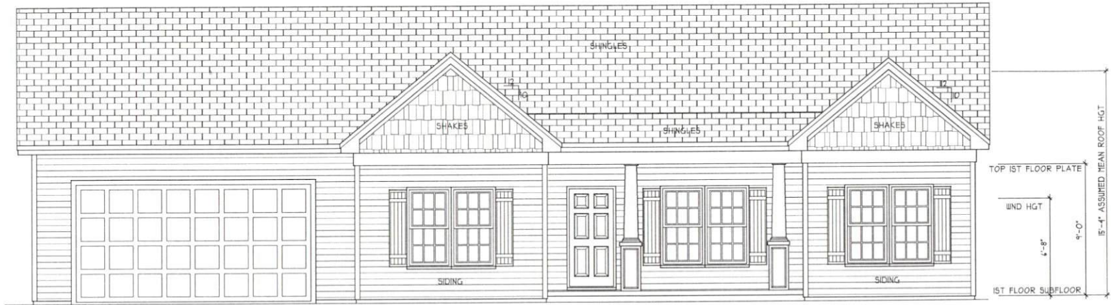
FRONT ELEVATION SCALE 1/4" = 1'-0"
