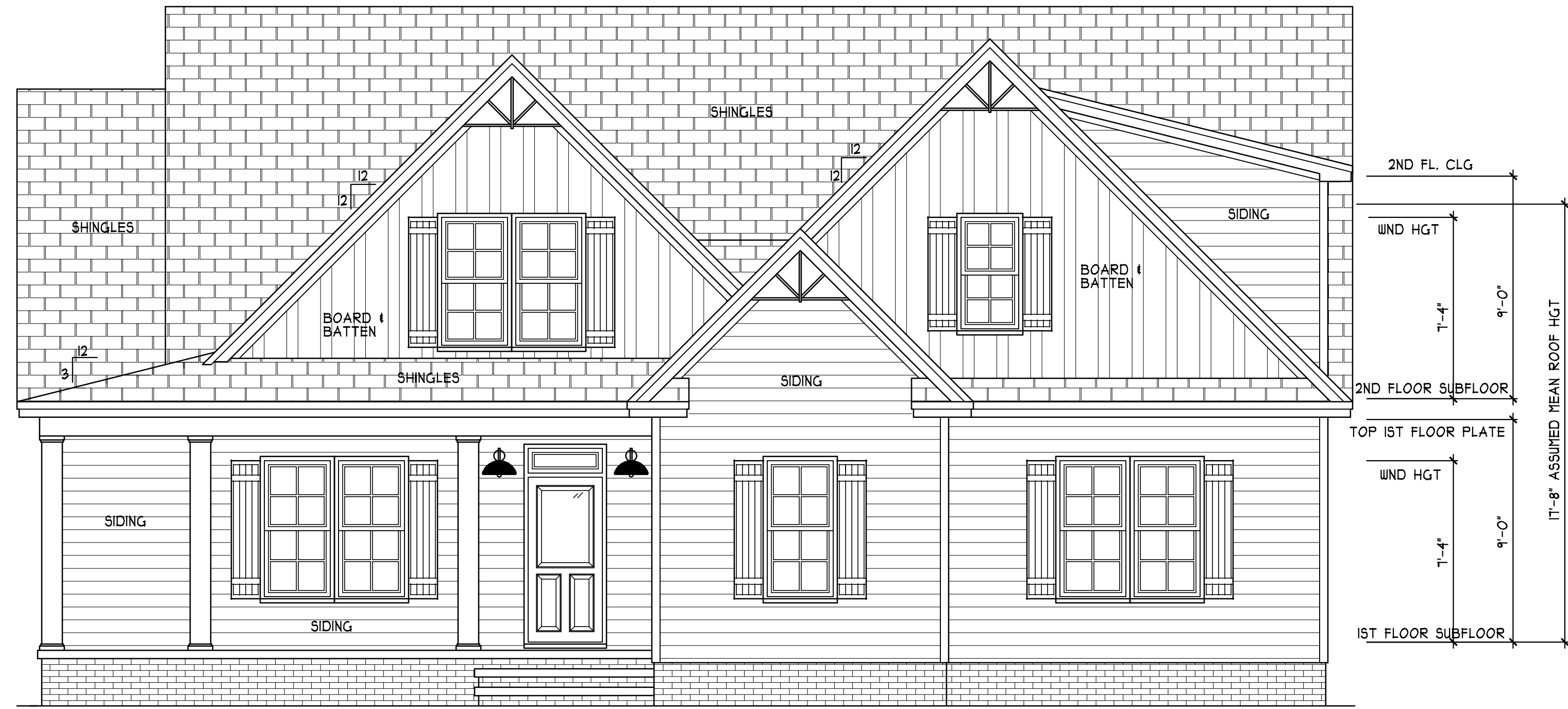
FRONT ELEVATION SCALE 1/4" = 1'-0"
