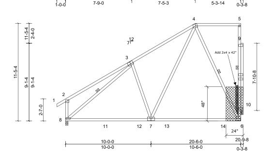
Repair for a section of the vertical missing between joints 6 and 10.
