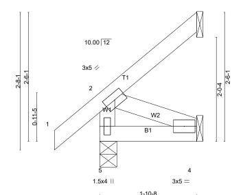
1-10-8 LOADING (psf) SPACING-CSI DEFL. 2-0-0 in (loc) I/defl L/d **TCLL** Ź0.0 Plate Grip DOL 1.15 TC 0.11 Vert(LL) -0.00 5 >999 240 (Roof Snow=20.0) вс Lumber DOL 1.15 0.03 Vert(CT) -0.00 4-5 >999 180 **TCDL** 10.0 Rep Stress Incr YES WB 0.03 Horz(CT) -0.00 3 n/a n/a **BCLL** 0.0 \* Code IBC2015/TPI2014 Matrix-MP BCDL 10.0
